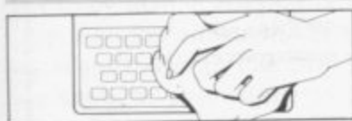
1. Make sure the original keyboard is clean and check that all the keys function.
